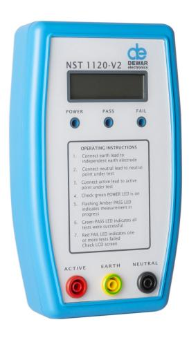
The Dewar Neutral Supply Tester (NST<sup>TM</sup>) measures volts, impedance and polarity in relation to the electrical grid supplies connected Active, Neutral and Earth to determine a safe or unsafe condition for industrial, commercial and domestic applications.
