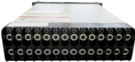
Each of these circuits is connected to a separate pair of terminals at the rear of the case, and comprises a contact which is normally closed when the protection device is in normal service.
