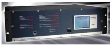
The TPU-1 universal teleprotection terminal is outstanding in its high level of modularity, allowing each user to obtain the services that best adapt to his requirements. Depending on the modules that make up the TPU-1 terminal, it can be configured to work with one or two transmission channels that can be either analog or digital. Furthermore, when working with two channels the terminal can be programmed to work as two independent teleprotection terminals.
